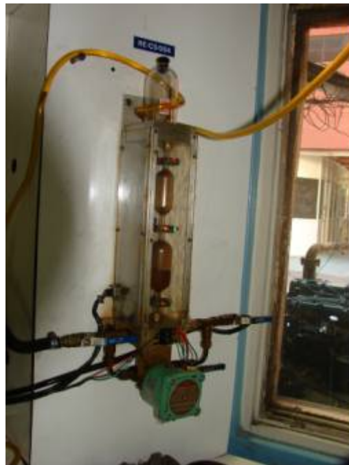
Figure 2.5 Measuring fuel consumption
