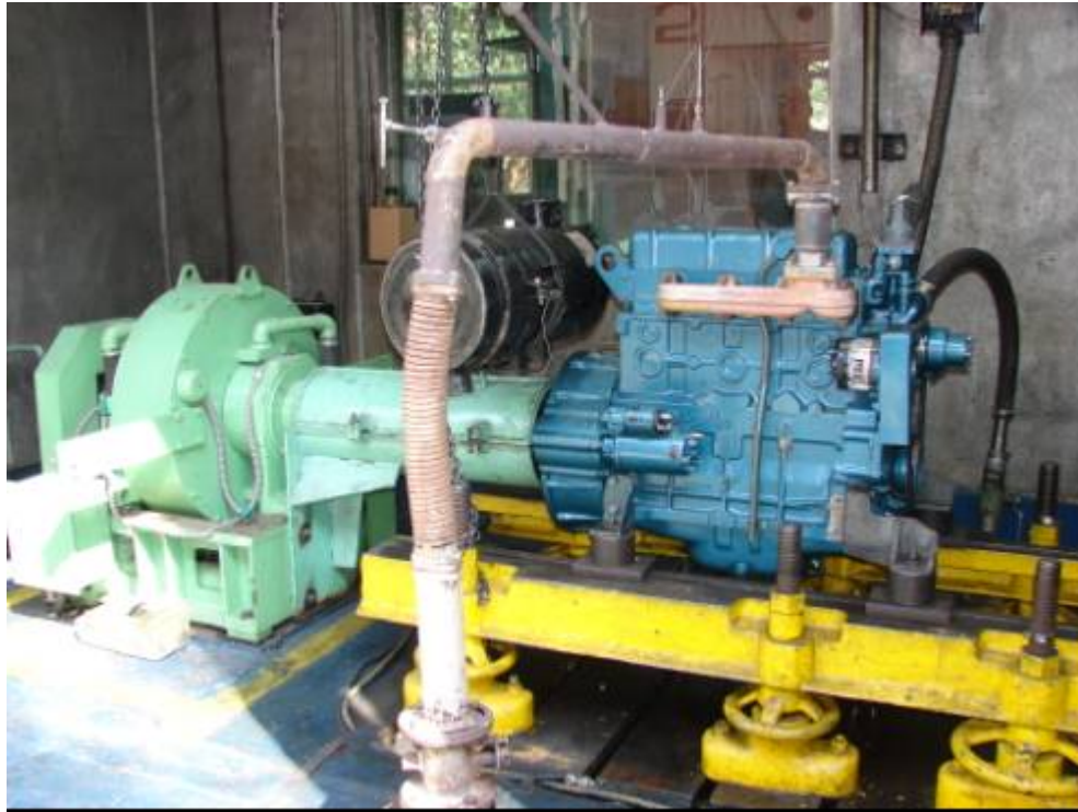
Figure 2.1 KOEL 4R1040NA on dynamometer
